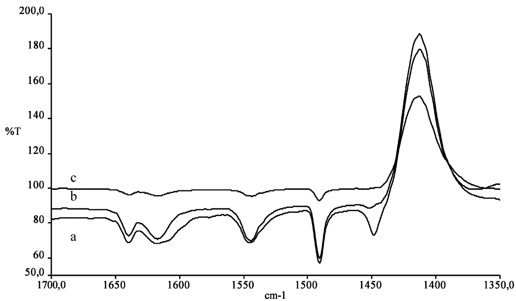
Fig. 4. Difference spectra of catalyst A after adsorption/desorption of pyridine at 21 (a), 100 (b) and 200°C (c).
